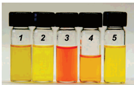
FIGURE 5. Colors of acetonitrile solutions of receptor 6 : (1) free macrocycle, (2) with \text{TBA}^+\text{Cl}^- , (3) with 1 equiv of \text{TBA}^+\text{HSO}_4^- , (4) with 1 equiv of \text{TBA}^+\text{H}_2\text{PO}_4^- , and (5) with \geq 2 equiv of \text{TBA}^+\text{H}_2\text{PO}_4^- .
